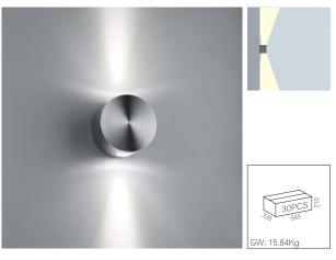
The product is made of pure aluminum and is molded through extrusion, and then shaped by CNC machines; the surface is varnished after brushing. Light transmission lens is made of PMMA material with transmittance rate as 93%, and the available angle options are 15°, 30°, 45°.
