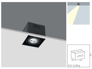
The face cover, inner ring and outer ring are made of aluminium alloy and shaped by extrusion; the main body box is made of cold rolled sheet; the surface is treated by dusting; LED light source is used; the radiation angle is adjustable and electric
