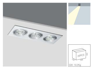
The main body parts are made of aluminium and then shaped by CNC machines; the surface is varnished after brushing; LED light source is used; the radiation angle is adjustable and electric
