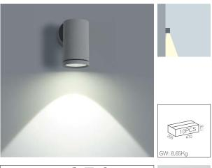
The cover and the lamp body are made of aluminum alloy and are molded through die-casting, and then shaped by CNC machines; the surface is treated by two processes of electrostatic dusting.
