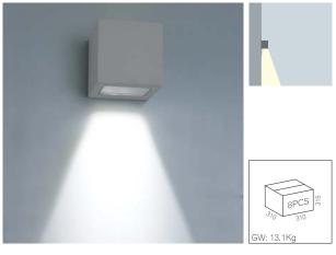
The lamp body is made of pure aluminum and is molded through extrusion. and then shaped by CNC machines; the surface is treated by two processes of electrostatic dusting.
